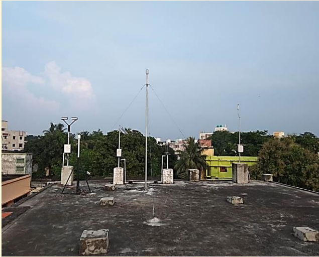
Instruments like rain gauge, electric field mill, lightning detector have been installed in Rampurhat College
